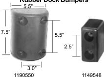
**Part No. 1190550 4 hole bumper** Molded, reinforced with flexible cord. Four 5/8" diameter mounting holes. 3<sup>3</sup>/<sub>4</sub>" deep, 5<sup>1</sup>/<sub>4</sub>" wide, 8" high.
